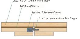
Slab Depression: Standard Profile Height 2-1/2" (64 mm)
