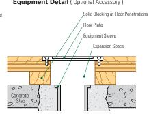
Standard Profile Height: 2 1/2" (64 mm) Optional Profile Height: 2 3/4" (70 mm)
